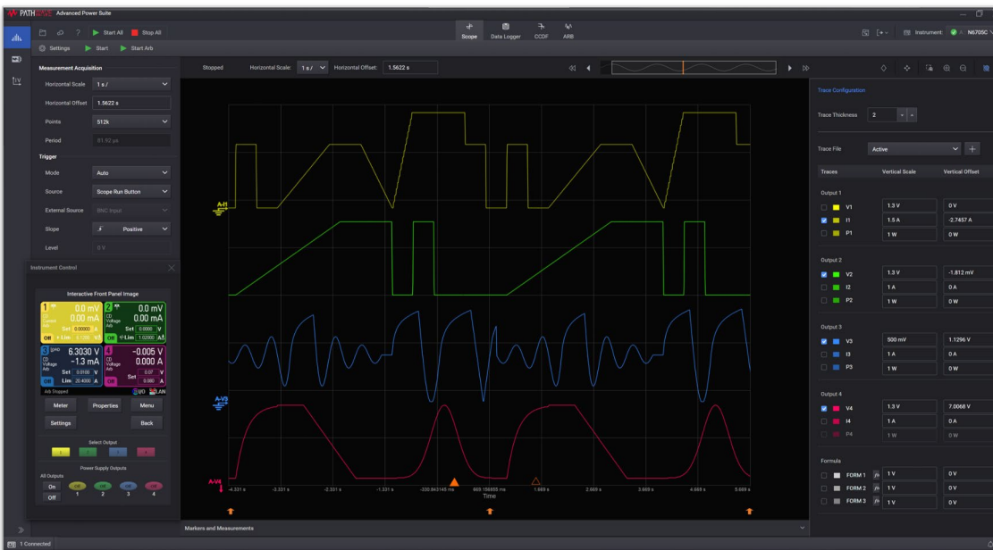
Figure 3. PW9252A interface with four channels connected
